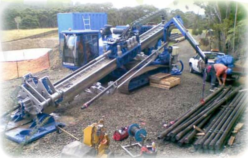
▲ Universal HDD Rig (100 ton pull back)
