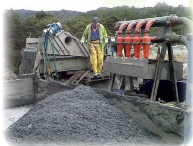
▲ Tunnel cuttings removed from the fluid with 3 shaker screens and 16 hydro cyclones
