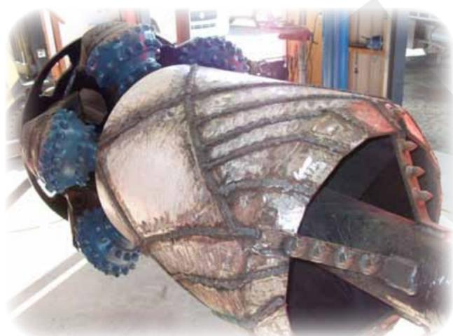
▲ 1050mm diameter tunnel requiring three reamer passes
